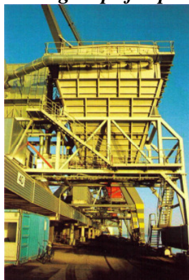
Figure 12: Hopper used by unloading ships for pellets and coal at the power plant
